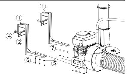
Attach the hanging brackets to the base with the hardware here
